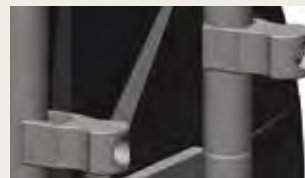
After the detent bolt has been removed, each handle may be folded outward
