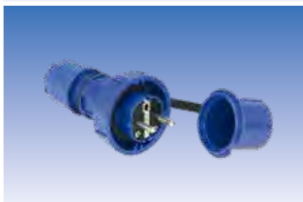
Plug with earthing contact, water-pressure-tight – with lock ring and cap – PC/ABS – DIN 49 443-R2 – IP66/68
