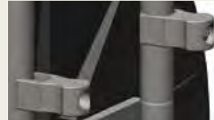
After the detent bolt has been removed, each handle may be folded outward
