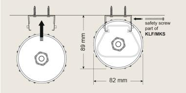
ACCESSORIES:Order No.2 pieces mounting clips<br/>with safety screwKLF/MKS2 pieces end-caps with<br/>cable gland M16 (cable<br/>diameter 5 - 10 mm)<br/>or<br/>cable gland M20 (cable<br/>diameter 6 - 12 mm)KLF/KAPSETM20
